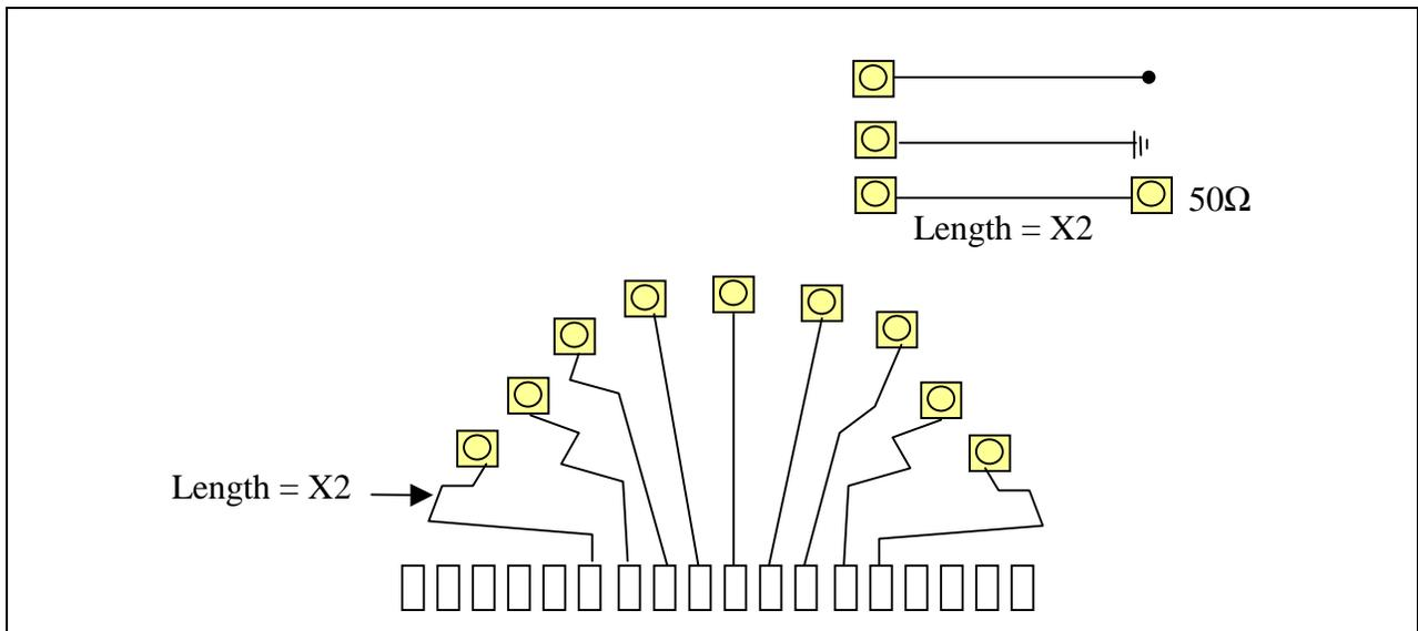
NOTE — Conductor traces are not made with sharp corners. They are only shown this way to illustrate designing equivalent length traces.
