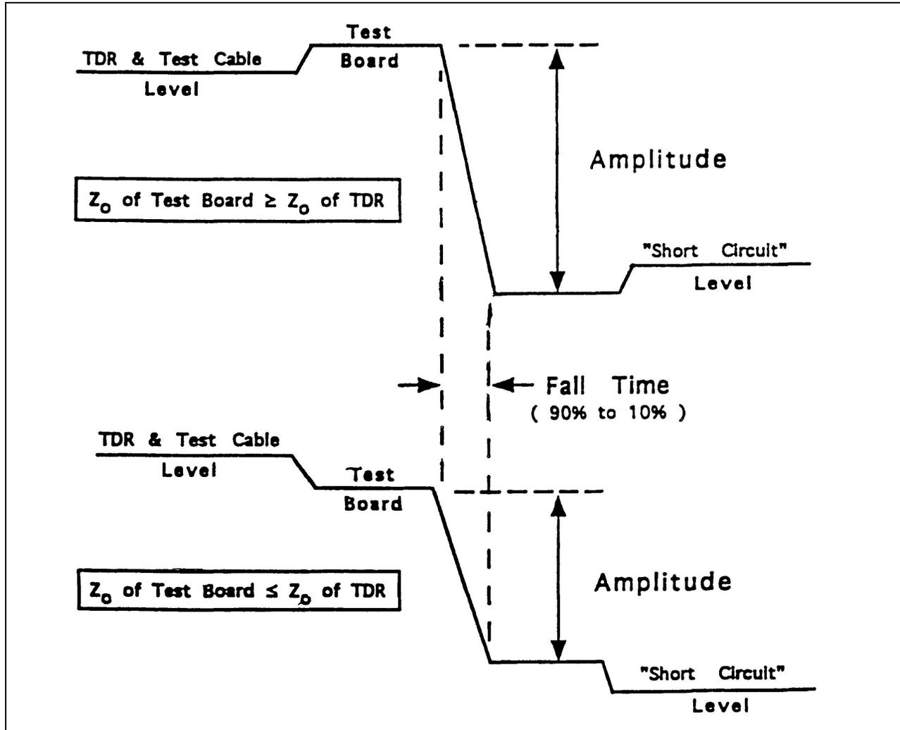
Figure C.3 – Example of near end reference trace
