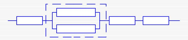
$$\omega_{21} = \frac{N_2}{r_{21}} = \frac{N_2}{F_{21} \bullet N_0} = \frac{F_2 \bullet N_0}{F_{21} \bullet N_0} = \frac{F_2}{F_{21}} \qquad R_S = \prod_{i=1}^n R_i = \prod_{i=1}^n (1 - \omega_{i(j)} F_{i(j)})$$
